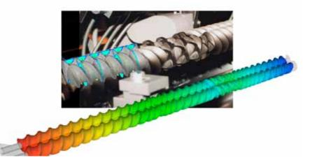
MST in Polyflow accounts for complex thermal and mechanical interactions for single- and twin-screw extruders.
