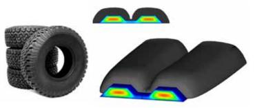
Polyflow's advanced numerics technology allows modeling of nonlinear behavior, such as velocity distribution in a die land and large die swell induced by stress relaxation in a tire application.
